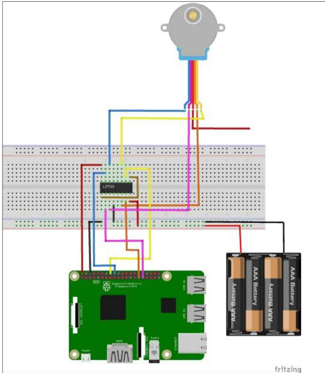
First, do all of your wiring BEFORE you power on the Raspberry Pi. We are working with an external power source, so you
