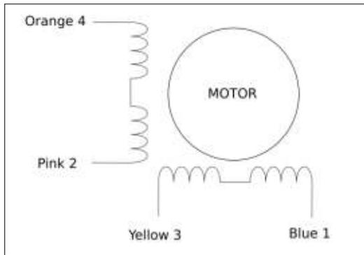
The numbers shown with the colors of the wires are for the 28BJY and yours may be different. The wire connector (if there is one) might differ from unit to unit. You can use an ohmmeter to verify the coils.
