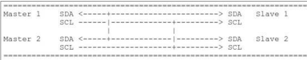
In the diagram above, SDA is the data line and SCL is the clock line.
