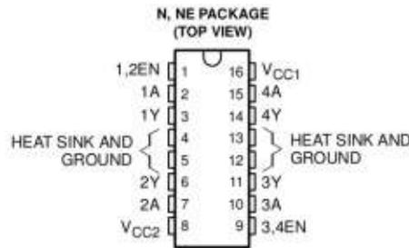
Pins 1 and 9 are enable pins. Think of these pins as an On/Off switch. A low state on the enable pin means the motor is off. A high state means that the motor CAN BE on. Let’s look at it as a logic table or truth table. Pins 1A and 2A are one side of the chip and are
