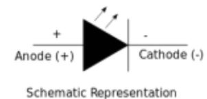
LEDs are Light Emitting Diodes and are the "standard" replacements for bulbs in just about everything. With a little care in design, they will last almost forever. An LED has two leads/wires called Anode and Cathode. The Anode is the positive
