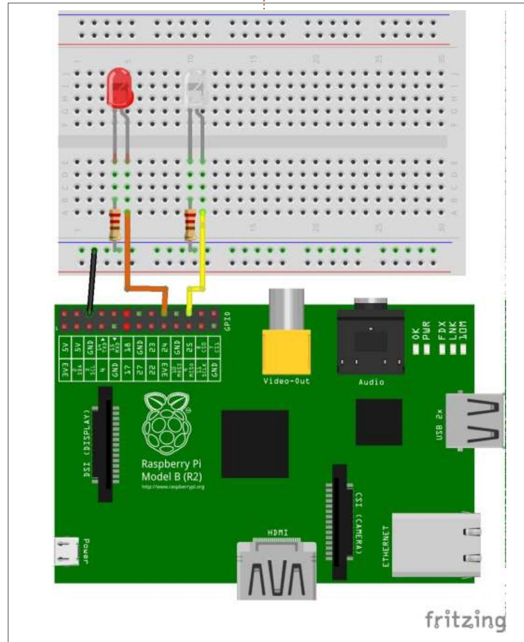
side of the LED is usually marked by the longer lead and the negative side is the one that has the flat spot on the base of the LED.
