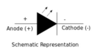
LEDs are Light Emitting Diodes and are the "standard" replacements for bulbs in just about everything. With a little care in design, they will last almost forever. An LED has two leads/wires called Anode and Cathode. The Anode is the positive
