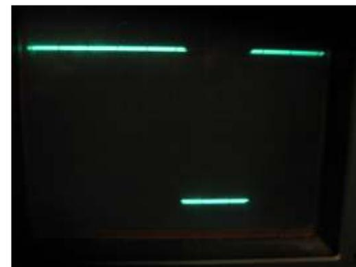
a bit from the 100% on all the time. As the program does its loop, it changes the duty cycle and makes the high longer or shorter depending on what part of the loop it is.
