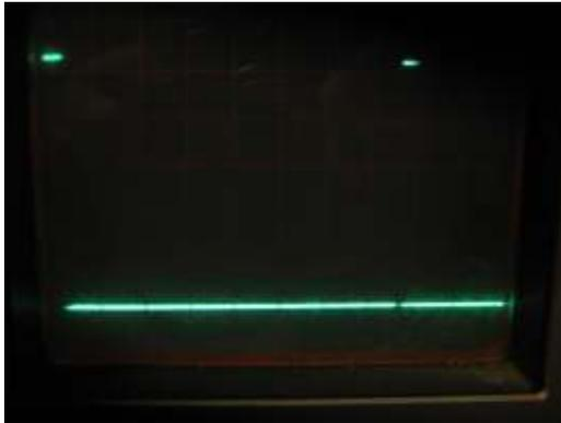
In the picture above, we have a duty cycle of about 5%. In this case the LED is turned on for such a short time, that it is extremely dim and for all intents and purposes it is off.
