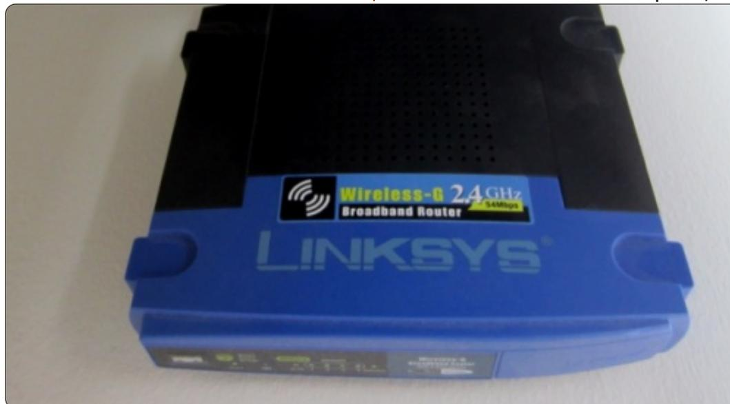
model supported. Linksys WRTGS v1 is supported by the tomato firmware as I write this article, but Linksys WRTGS v5 is not supported. You have to be careful, because even slight differences could mean you're left with a doorstop instead of a router.
