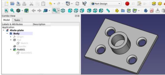
Note, on the left we have (below Chamfer) a new Pad and new Sketch. They only apply to the pipe socket.
