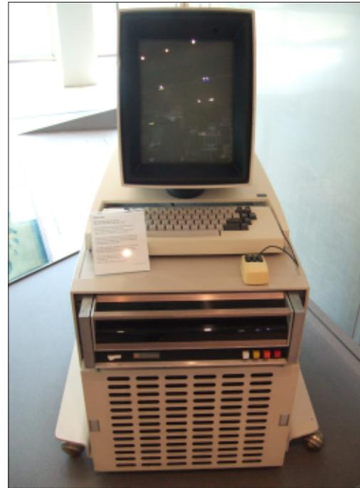
Some argue that Alto is the first personal computer, while others say it was a small Minicomputer. In either case, it was quite a machine for its day. It used a TTL-based CPU at 5.88 MHz, with 128 kilobytes of memory, 2.5 MB cartridge (like hard drive storage), 606 x 808 resolution monitor, keyboard, 3-button mouse, 5-key chorded keypad, and Ethernet.
