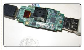
What is it? A fully functioning linux box the size of a USB stick. HDMI: check. USB: check (well, one port, anyway). 700MHz ARM11 processor with 128MB of memory: check. With storage available through an SD card slot, this thing has everything you could want in a computer (except maybe Wi-Fi; at the time of this writing I was unable to confirm networking), and you can carry it on your key-chain.
