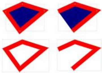
The obvious take-away from this is that 0.92 removes the fill entirely before the stroke is converted to a path. I've shown both closed and open shapes to make it clear that the behaviour is the same in both
