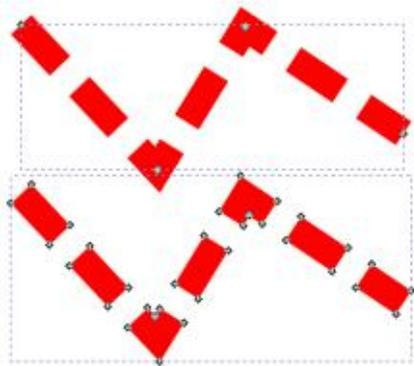
Our converted line is starting to look a bit more interesting. Instead of a simple filled path, we now have a complex path, consisting of a number of filled sub-paths which match the visual appearance of the original line.
