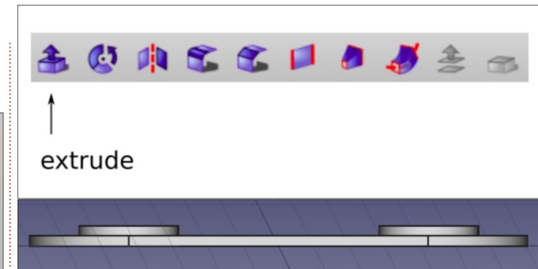
Now do the same with the other circle, converting it also into a cylinder 4 mm high. Finally, let us make an extrusion from the Wire piece, but this time only 2 mm high.
