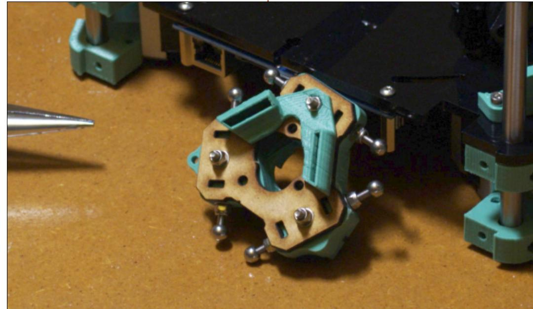
screwed in place. You might need a metal file for this to shorten the screws and bring the steel balls back a touch.
